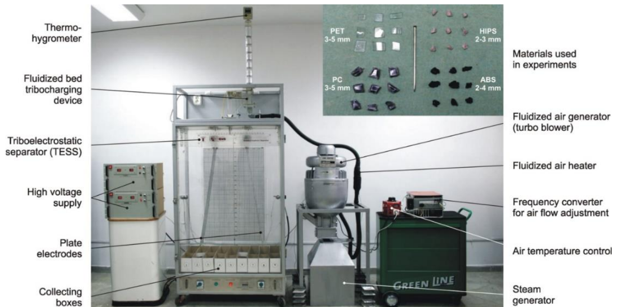
FIGURE 8. Experimental set-up of the laboratory free-fall triboelectrostatic separator used for plastic waste separation.
