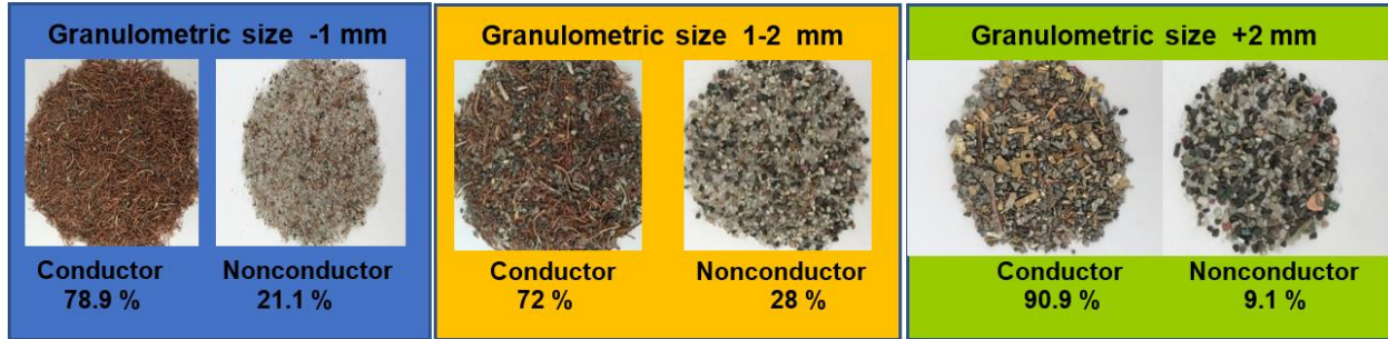
FIGURE 4. Results of the corona-electrostatic separation of the Cu/Al/glass/plastic mixture.
