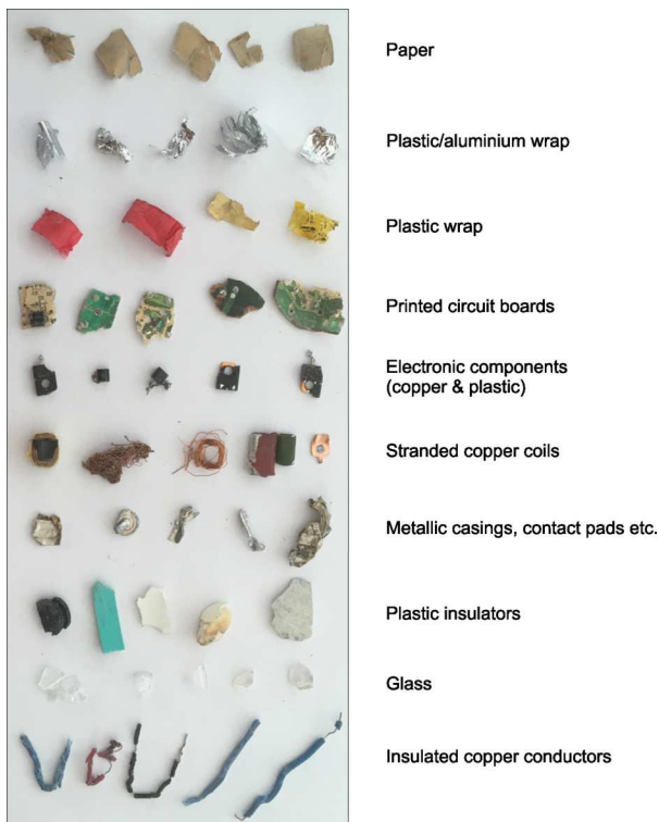
Fig. 2 Components of the granular waste obtained from the recycling process of WEEE after the first shredding operation with a 20 mm sieve.
